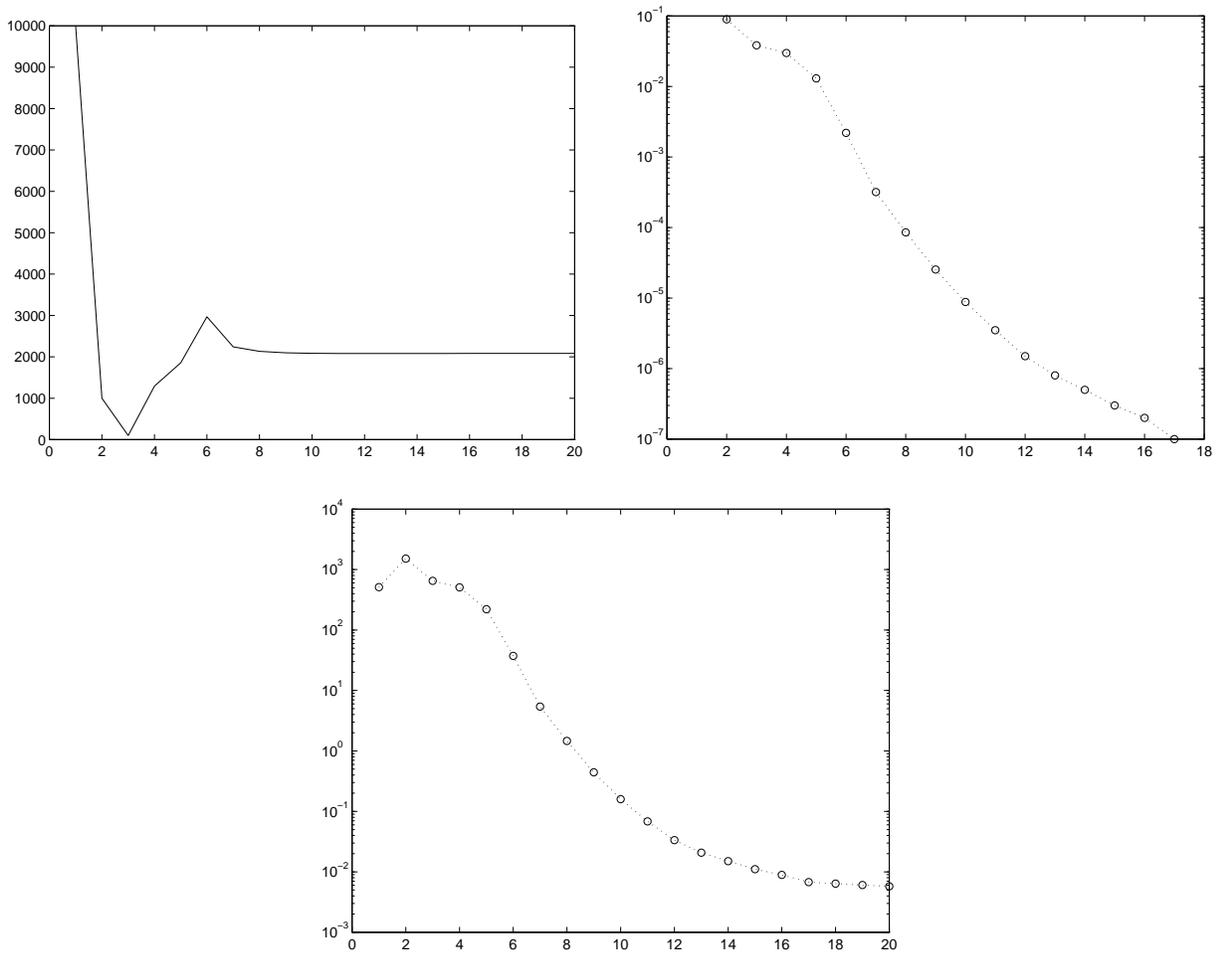
Fig. 4. **Upper-Left:** The regularization parameter,  $\lambda$ , as a function of the number of iterations. **Upper-Right:** The residual of the constraint, *e.g.*  $N(u, \lambda)$  as a function of the iterations. **Center:** The residual of the coupled  $(G, N)$  system. Again,  $\lambda$  is quickly identified, and the convergence is linear as expected.
