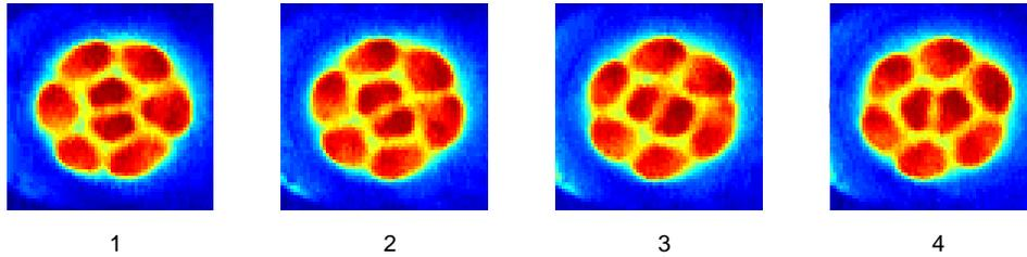
FIGURE 14. Snapshots from a counter-rotating rings state in the combustion experiment.
