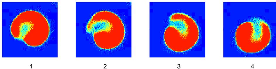
FIGURE 2. Evolution of a single-cell flame from a combustion experiment. The algorithm of Section 3 identifies this pattern as a MRW with average drift  $\omega_r = 22.6726 \text{ rad/sec}$  and frequency of modulations  $\omega_m = 23.1938 \text{ rad/sec}$ .
