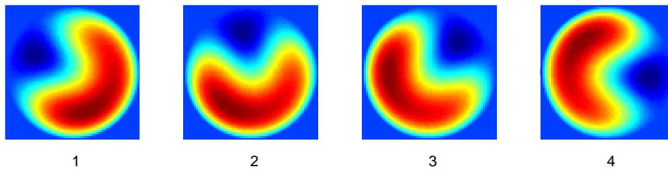
FIGURE 1. Evolution of a computational rotating wave simulating a single-cell flame in the combustion of premixed gases. The cell rotates uniformly and without changing shape.
