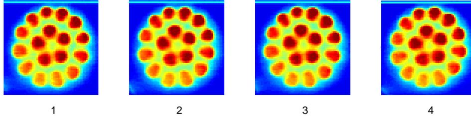
FIGURE 18. A ratcheting experimental state: the outer ring slowly drifts counter-clockwise with punctuated periods of abrupt, faster angular displacements. The inner rings remains stationary with distinctive  $\mathcal{D}_5$  spatial symmetry (symmetry of a pentagon).
