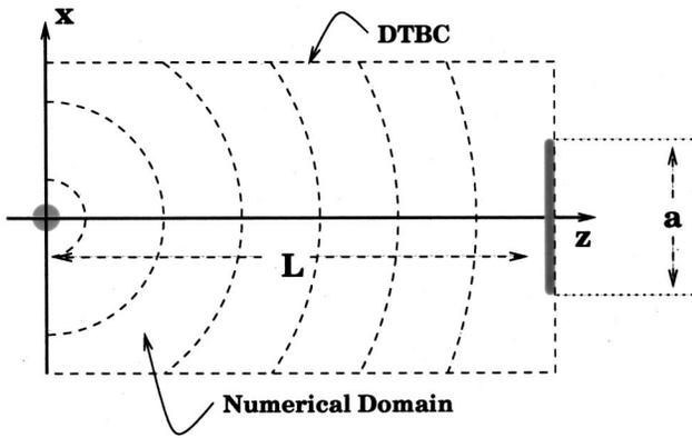
FIG. 1. Setting for time-reversal acoustics. A point source emits a wave, which is received on a screen of width  $a$ —the *time-reversal mirror* (TRM)—at a distance  $L$  from the source. The domain of numerical solution of the (parabolic) wave equation is shown with a dotted line, and DTBC stands for *discrete transparent boundary conditions*.
