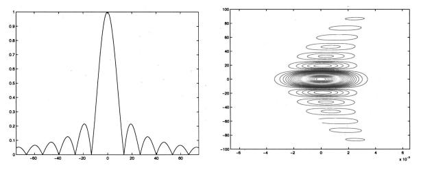
FIG. 3. The left figure shows the spatial diffraction pattern of the amplitude of (25) at time t=0. The right figure is a space-time contour plot of the amplitude of (25) and shows the parabolic shift in arrival time. Here, the pulse width is  $\sigma_t = 1.33$  ms, the TRM width a = 50 m, the propagation speed is  $c_0 = 1500$  m/s, the propagation distance is L = 1000 m, and the period of the carrier is 0.22 ms at 4.5 KHz.
