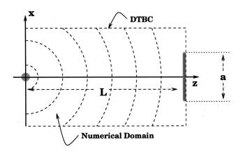
FIG. 1. Setting for time-reversal acoustics. A point source emits a wave, which is received on a screen of width *a*—the *time-reversal mirror* (TRM)— at a distance *L* from the source. The domain of numerical solution of the (parabolic) wave equation is shown with a dotted line, and DTBC stands for *discrete transparent boundary conditions*.
