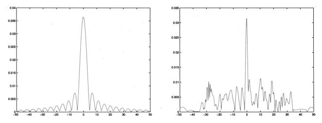
FIG. 15. Homogeneous medium on the left, random medium on the right. Type of boundary conditions: *DTBC* with TRM width 60 m. We can clearly see super-resolution as the recompressed peak is narrower in the random medium case. The fluctuations in the sidelobes are partly due to the fact that we are pushing the paraxial approximation beyond its limit; the 10% contrast is stretching the "low-contrast" assumption.
