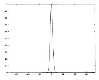
FIG. 4. The spatial shape of the compressed pulse with a Gaussian aperture function at time t=0, from (31). Here, the pulse width is  $\sigma_t = 1.33$  ms, the TRM width is a = 50 m, the propagation speed is c = 1500 m/s, propagation distance is L = 1000 m, and the time period of the carrier is 0.22 ms. Note the absence of Fresnel zones for a Gaussian TRM.
