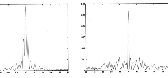
FIG. 16. Homogeneous medium on the left, random medium on the right. Type of boundary conditions: *Waveguide* with TRM width 60 m. The waveguide effects are quite strong, but an argument for super-resolution can be made, since the peak is better defined. Randomness does not, in any case, degrade the results.
