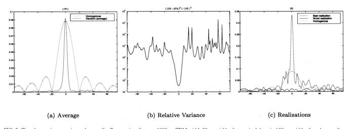
FIG. 2. Time-harmonic waves in random media. Propagation distance 1000 m, TRM width 50 m, width of numerical domain 150 m, width of random medium 112.5 m, contrast  $\pm 5\%$ , 428 realizations. (a) Amplitude of the mean: Homogeneous (light) and average over random realizations (dark) case. (b) Relative variance, >O(1) except for a very small interval. (c) Individual realizations that show super-resolution (high) as well as no resolution at all (low).
