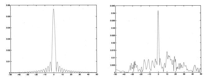
FIG. 13. The recompressed pulse for homogeneous (left) and random (right) media. The propagation distance is 800 m, the domain width is 100 m, and the maximal contrast is 10%. The boundary conditions are: *DTBC*. TRM width 100 m. Here, we can clearly see super-resolution as the recompressed peak is narrower in the random medium.
