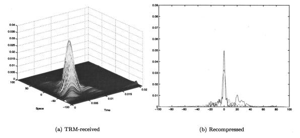
FIG. 8. In this simulation the propagation distance is 600 m. Now, we clearly see the super-resolution phenomenon: the peak of the recompressed pulse in the random medium (upper) is sharper than the one for the homogeneous medium (lower). (All other parameters are as in Fig. 7.)
