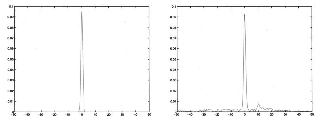
FIG. 14. Homogeneous medium on the left, random medium on the right. Here, we have *Waveguide* boundary conditions with TRM width 100 m. We capture all the energy inside the waveguide on the TRM, so the waveguide effect is much stronger than the random-medium effect. There can be no super-resolution in this setting.
