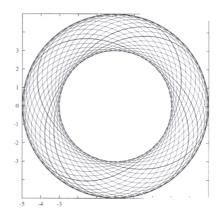
**Figure 2:** Forward trajectory of an unperturbed spherical pendulum projected on the xy-plane.
