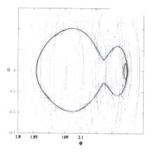
**Figure 7:** Magnification of Figure 6. A periodic orbit is found embedded in the chaotic attractor.
